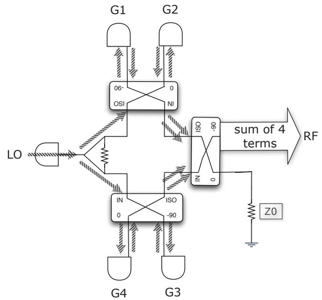
Figure 8: linear combination at RF
