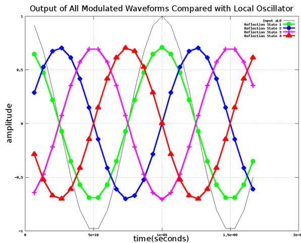
Figure 14: all four modulated output waveforms compared against the LO.
