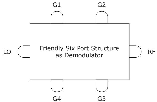
Figure 15: six-port as demodulator
