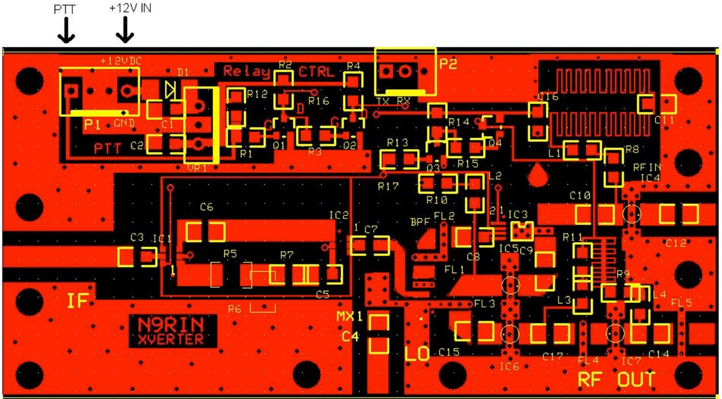
Figure 1: N6RIN 3.4GHz Transverter
