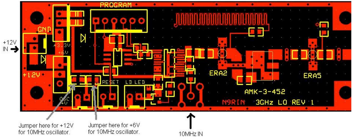
**Figure 2: 3GHz Local Oscillator**
