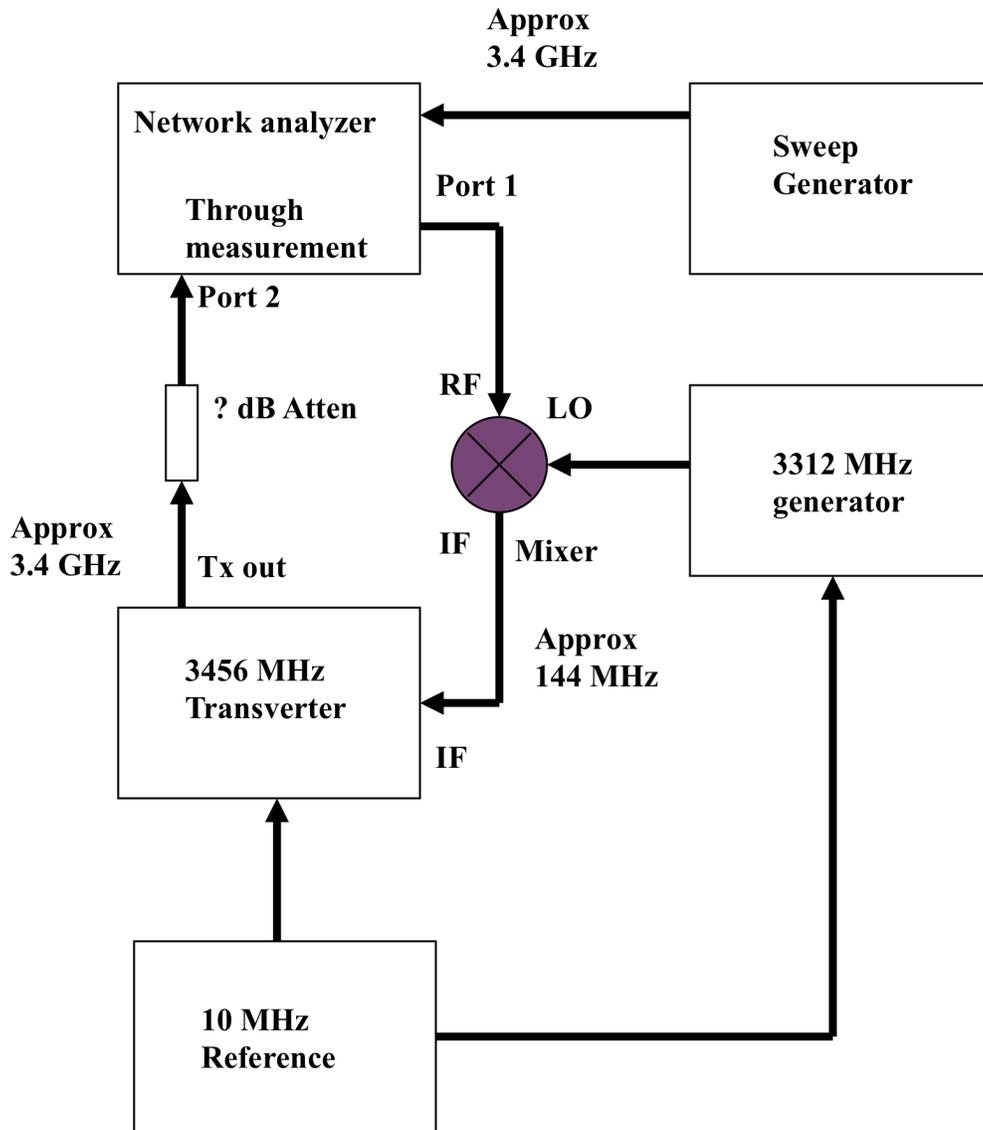
Figure 4: Transverter Transmit Amplitude and Phase Measurement Setup
