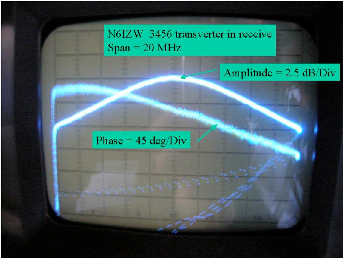
**Figure 6: Test Setup Plot of Amplitude and Phase Over 20MHz Span**
