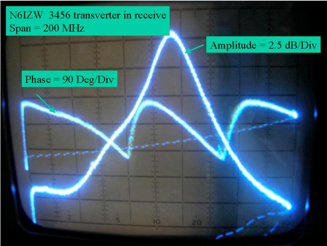
**Figure 5: Test Setup Plot of Amplitude and Phase Over 200MHz Span**
