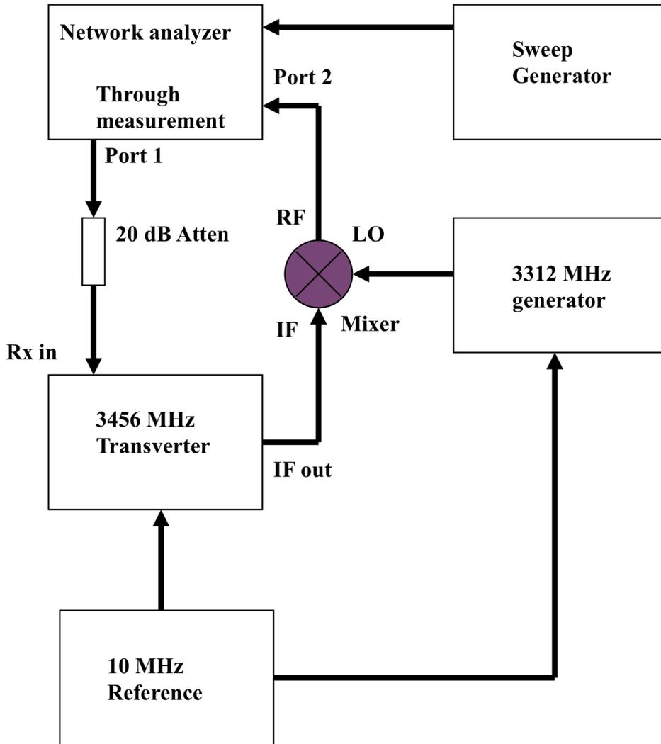
Figure 3: Transverter Receive Amplitude and Phase Measurement Setup
