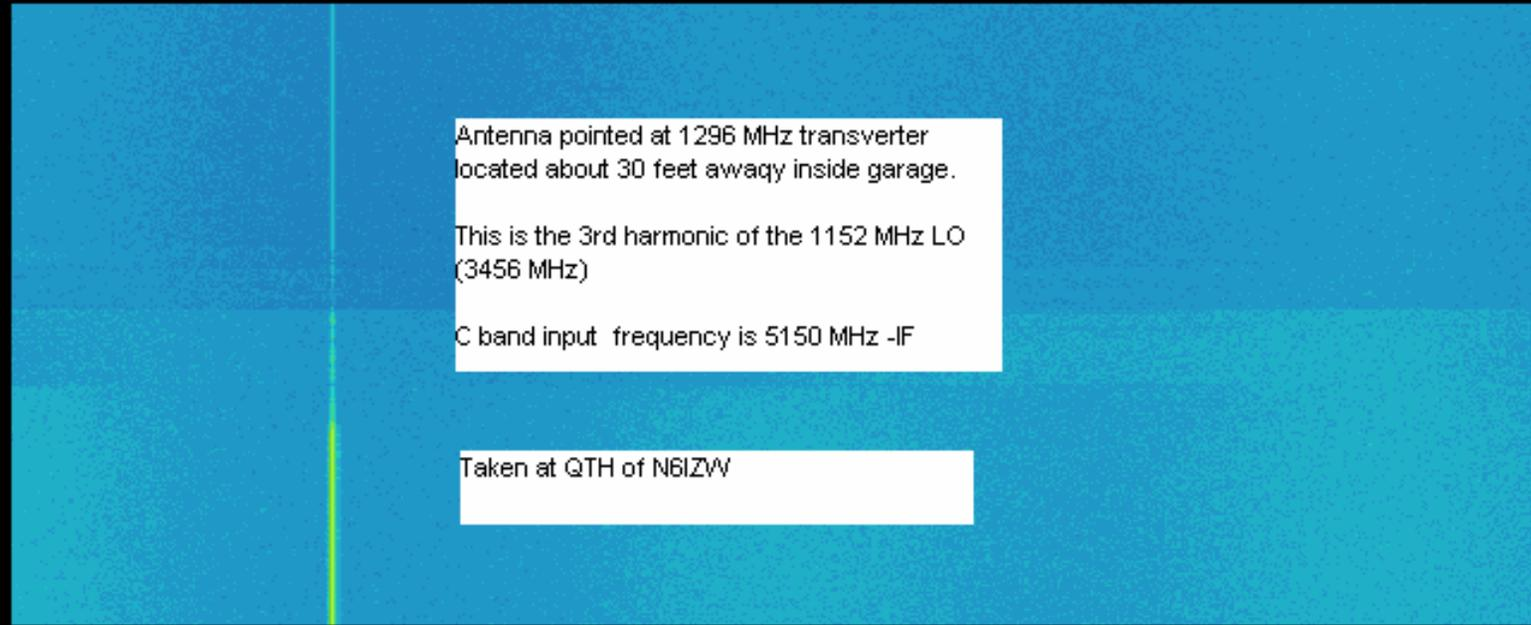
Antenna pointed at 1296 MHz transverter located about 30 feet away inside garage.
