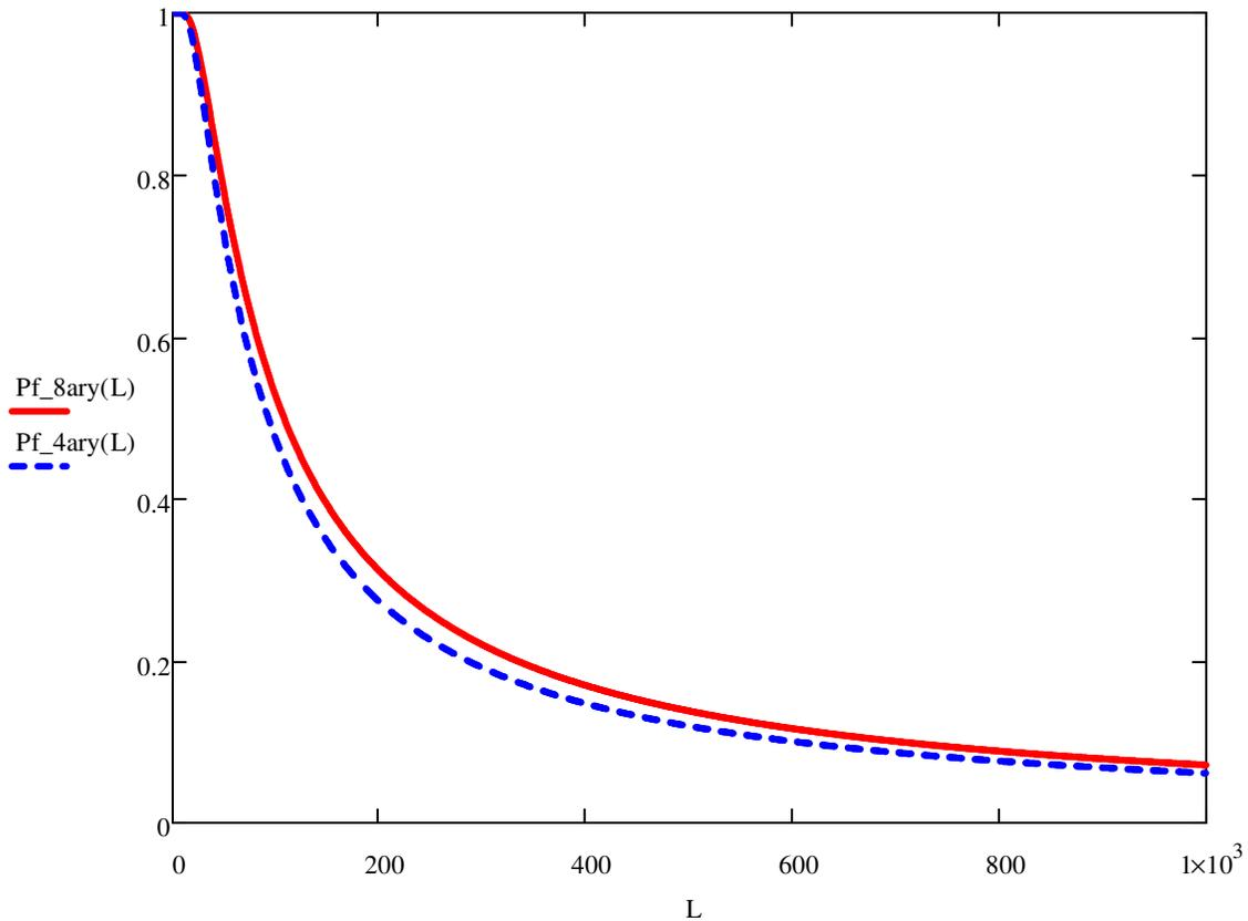
This shows the effect of adding new channels to an FH-8ary FSK system with 85 independent users transmitting random data. The probability of collision decreases rapidly and then flattens out.
