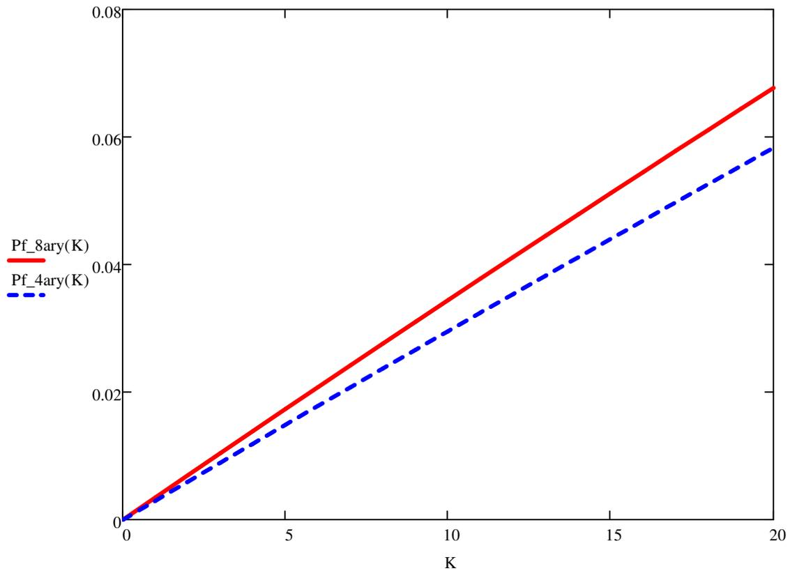
Probabilities of collision range from 0.7% for 2 users to 6.8% for 20 users (8-ary FSK).
