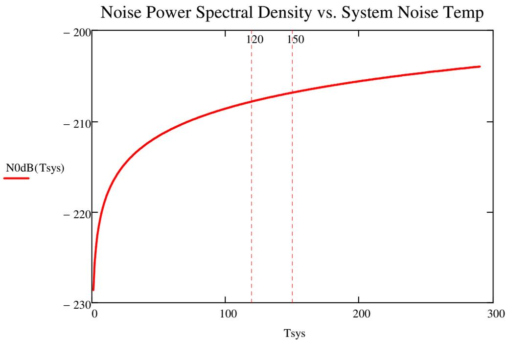
Receive noise temperature in the expected range of 120K to 150K gives the following spectral noise densities in dB.
